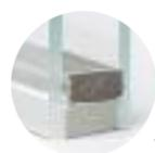
The optional Foam Spacer System is unique in its patented design. By combining a structural foam spacer with a seal of hot melt butyl to create a non-conductive edge, the non-metal Foam Spacer System eliminates any metal to glass contact, thereby increasing the edge of glass temperatures by over 16 degrees, which proves to be over 60% more energy-efficient than a traditional box-shaped spacer.
