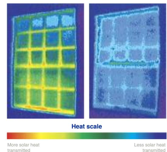
undetectable metallic coating to the second surface of an insulated glass unit. This coating helps to block heat gain in the summer while retaining furnace heat and allowing warm short wave solar rays in the winter.
